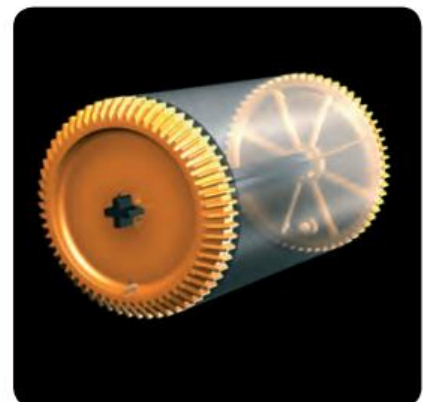
The pair of wheels acts like a roller with a small contact surface. The force of friction, as you know, is independent of the size of the contact surface.
