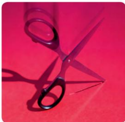
A pair of scissors consists of two levers. Their cutting force increases as you get closer to their shared pivot point.
