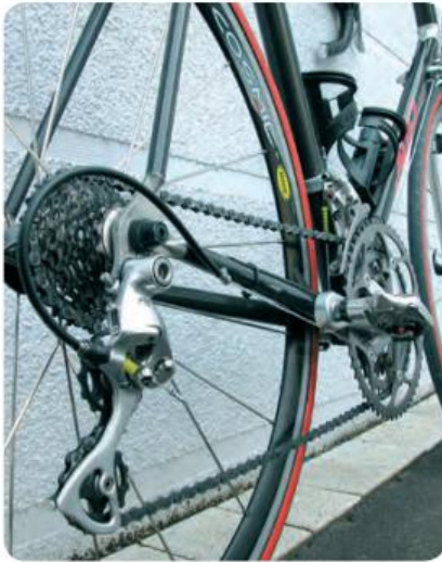
A bicyclist can use a gearshift to adjust to the hills of a street. The transmission system allows the force on the pedals to be kept fairly constant.
