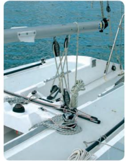
The fixed pulleys on sailboats spare you tedious distances and cumbersome handles.
