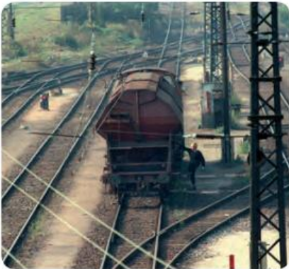
A railway hump yard uses a slight slope to switch a car to one track or another.
