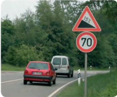
The sign indicates that the road will drop 1.5 m over a distance of 10 m.
