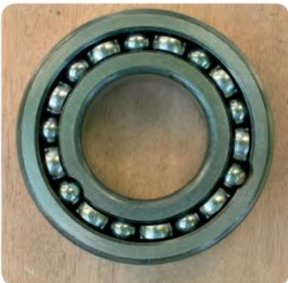
Minimal friction loss in a ball bearing.
