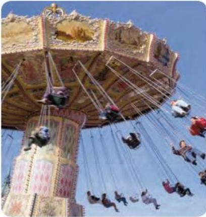
The same goes for an amusement park swing ride: the faster it spins, the farther up and out the chairs fly.
