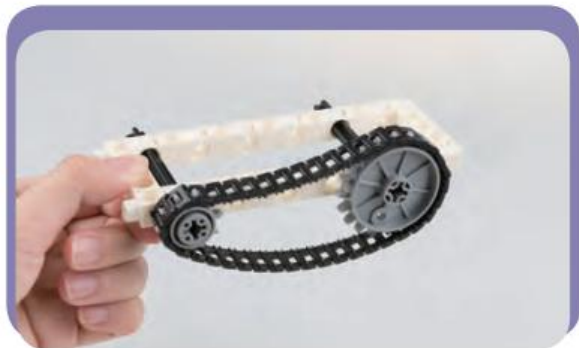
鍊條組裝成品須有垂墜感，可加減一個鍊條去做調整 The gear chain should be a little loose when used to connect two chain gears. A unit chain can be added or reduced to adjust the tightness.
