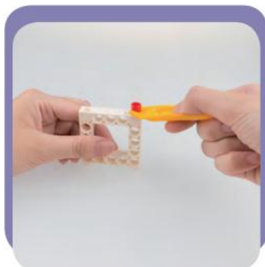
長結合鍵拆解法 Pull Peg off Frame with side A of Peg Remover.
